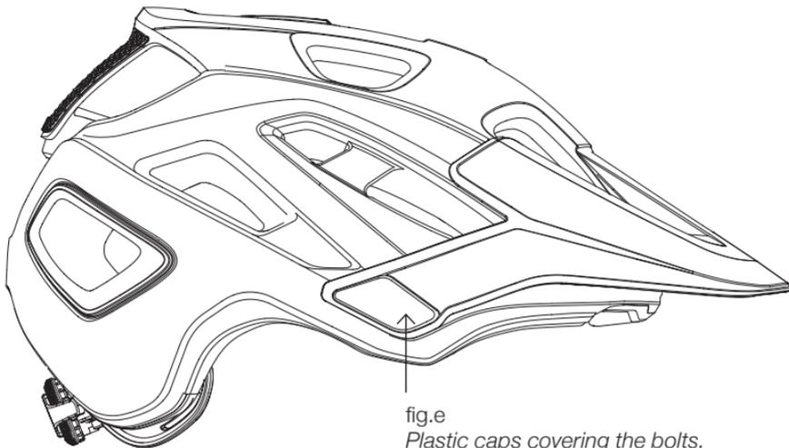
Jackal KinetiCore has an adjustable visor secured to the helmet by 2x metal bolts. These bolts are covered by plastic caps to retain the clean aesthetic of the helmet. If the bolts loosen, for example after lots of vibration due to riding hard on rough terrain, it may be necessary to tighten them.
